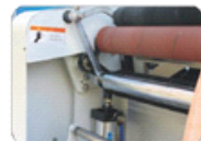
气动式海绵压床配置 Pneumatic System For Pressing Foams
